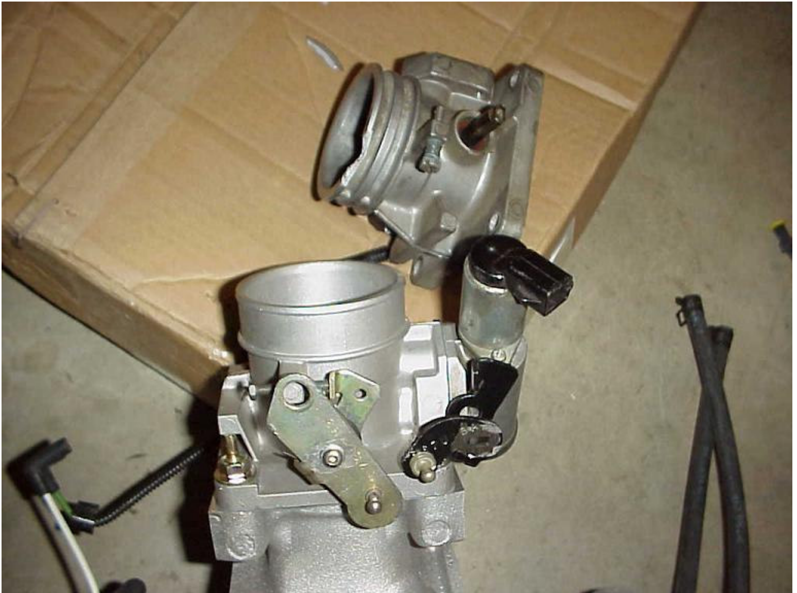
This one shows the Explorer t/b and the donor Mustang t/b, after its bellcrank was removed. The Explorer bellcrank is sitting next to the grafted on Mustang bellcrank
